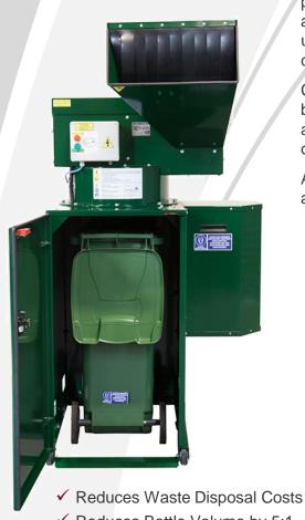
This Volume Fed bottle crusher can crush up to 4000 bottles per hour or 680 bottles in 10 minutes and can be used indoors and outdoors. The built-in extraction system makes it ideal for use in areas with restricted ventilation. Waste glass is collected in a 140L wheelie bin located inside the machine.
